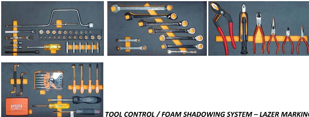
TOOL CONTROL / FOAM SHADOWING SYSTEM – LAZER MARKING
