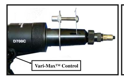
The **D-700-VM Vari-Max**<sup>™</sup> feature enables the user to set a pull force when upsetting a blind rivet nut or insert to help insure a proper installation without damaging the threads of the blind nut insert or the threads on the pull-up stud. The normal operating range for the D-700-VM is 600 to 5,000 lbf. The Vari-Max<sup>™</sup> is located on the tool on the side opposite the release button (right side of the tool facing forward).
