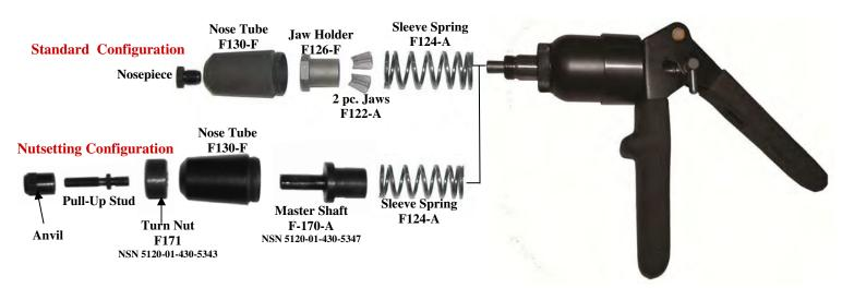
**NOTE:** Space is provided so that a Cherry-Max® Offset, Right Angle and Extended Straight Pulling Heads may be added as needed. The D-100-MIL-1 is supplied in a weather tight metal carrying case (2 1/2" x 6 1/2" x 10") along with operating instructions, parts list and warranty card.
