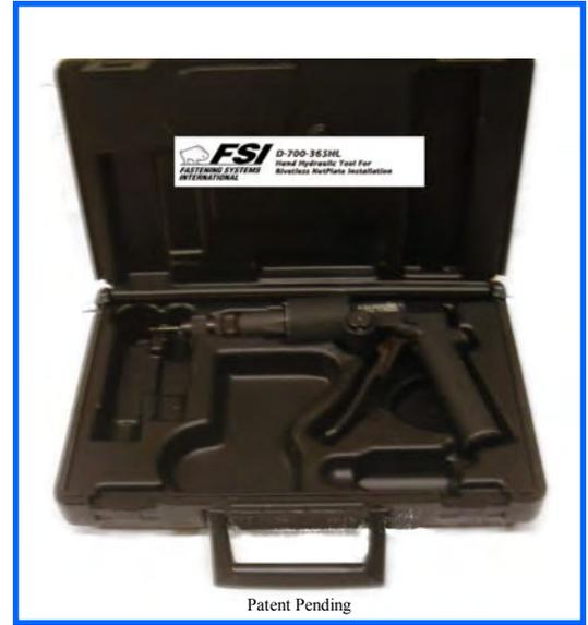
**D-700-365HL Rivetless Nutplate Tool Kit**
