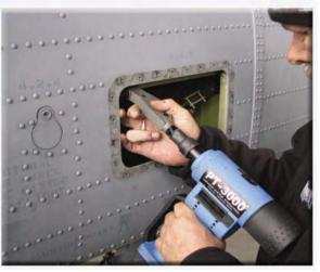
(unthreading) of the head during the positioning and re-positioning process. Available for use with Cherry Aerospace, Huck, and Olympic style offset and right angle pulling heads, these adapters provide a major improvement in flexibility with negligible changes in adapter profile and weight. Made in the USA.
