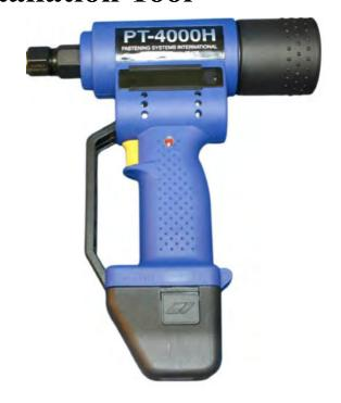
EACTING TO THE NEED FOR A VERSATILE, CORDLESS RIVETER AND LOCKBOLT INSTALLATION TOOL that uses conventional aerospace pulling heads, FSI is pleased to offer the PT-4000H. Eliminating trip hazards from air hose while providing positive FOD control, the 12 VDC Battery operated PT-4000H affords the sheet metal technician true portability.
