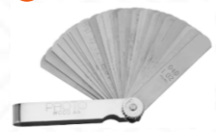
PN CODE J000AA DESCRIPTION 25 Blade Master Feeler Gauge Set (0.0015" to 0.040" except 0.019")
