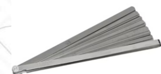
PN CODE J000TL DESCRIPTION 25 Blade Long Feeler Gauge Set (0.0015" to 0.040")
